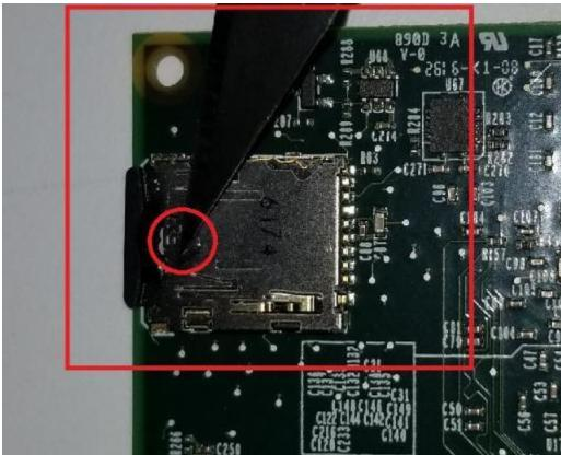
d. Use caution to not damage the socket or other parts of the CPU board.
