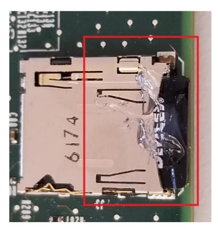
i. Set the CPU aside for about 20 min to allow the RTV to harden. It will not become completely hard and may be a bit tacky to the touch. This is ok and it will completely dry in the unit.
