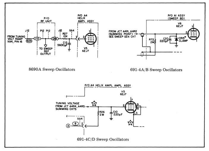
Figure 1. Partial schematics of Helix Amplifier Modification
