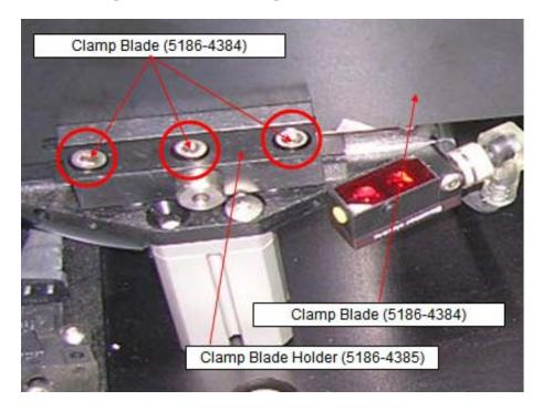
**Step 2.** Unscrew M5 x 12 countersunk x 2pcs using Allen Key (Metric, 3mm)
