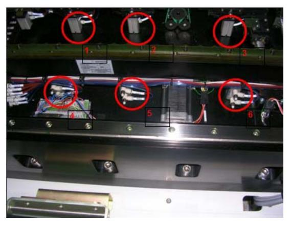
**Step 5.** Adjust air restrictor so downstroke of clamps is dampened sufficiently so as not to disturb Pre reflow components.
