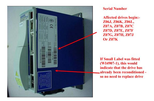
Example of reconditioned drive – this has old serial number, but also has rework label (WI4907-1) as shown on the bottom right corner
