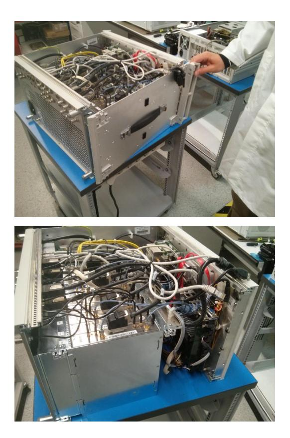
© Keysight Technologies 2015-2016 Modification Recommended Service Note Version 1.2 | January 28, 2016| Page **3** of **5**  Check that the RAM modules are secured with hot melt glue as shown in the following pictures:
