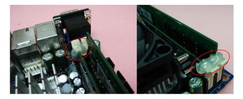
The glue must be applied all the way down from the locker to the memory slot, and both RAM modules must be tied together (i.e. building a "bridge" between the latches).
