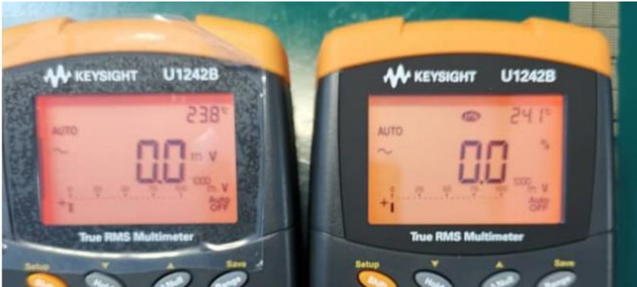
Left: New backlight color (600nm) Right: Original backlight color (598nm)
