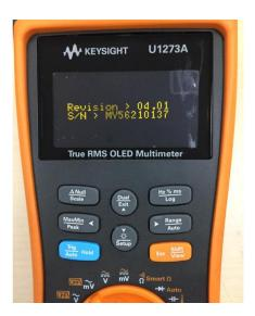
5. Firmware version 3.02 and 4.01 will resolve the incorrect DCI measurement value when using average measurement mode.
