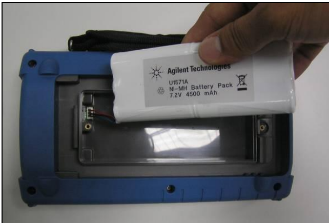
Figure 4 Unplug the 3-wire connector from the PCBA board using a tweezer.
