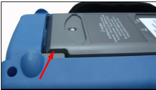
Figure 1 Push towards the arrow direction to remove the stand
