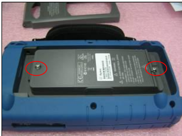
Figure 14 Tighten the 2 screws
