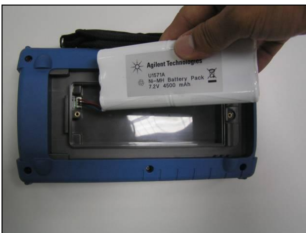
Figure 13 Reconnect the battery
