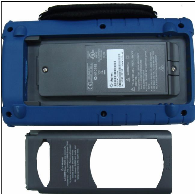
Figure 2 Disassemble the stand from the instrument
