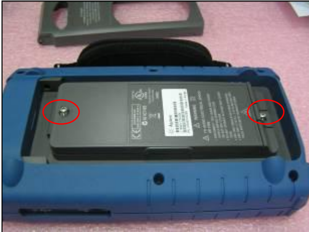
Figure 3 Remove battery cover screws
