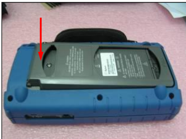
Figure 15 Press the rear stand in the direction of the arrow
