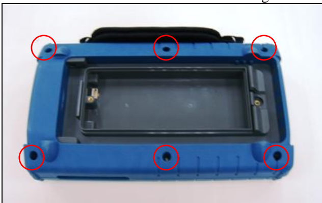
Figure 5 Remove the screws from the rear casing
