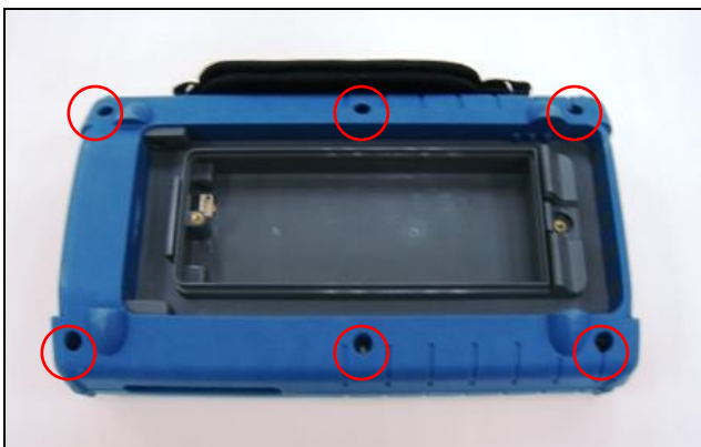
Figure 12 Fasten the screws
