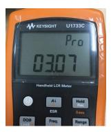
5. Firmware revision 3.07 will resolve the incorrect resistance measurement value when measuring below  $7M\Omega$  on  $20M\Omega$  range.
