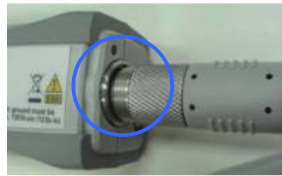
Figure 2: USB power sensor cable not fully attached to power sensor unit
