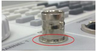
a) BNC connector not securely tightened
