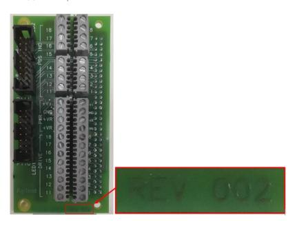
2. Perform continuity test using a multimeter at the bottom of PCA between terminals 7 to 17, and terminals 8 to 18, as shown in the figures below.
