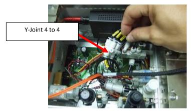
Figure 21: Identifying the tubing with Y4.2.C
