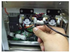
Figure 20: Plugging the M6 tubing end
