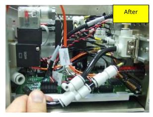
Figure 6: Disconnecting M8 tubing end from the Pilot Valve
