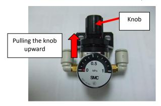
Figure 33: Pulling the knob upwards
