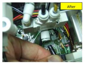
Figure 7: Disconnecting M6 tubing end from the Air Pilot Valve
