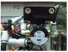
Figure 36: Pressure Regulator at P2 operating at 0.22MPa
