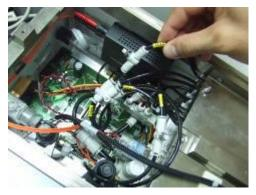
Figure 27: Plugging in theM4 tubing end with the label of Y4.3.B into the inline flow controller B
