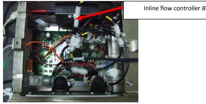
Figure 39: Gradually loosening the knob of the inline flow controller B
