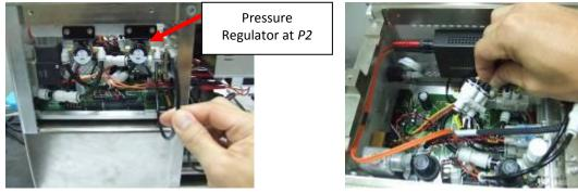
Figure 24: Identifying the M4 tubing end and make connection accordingly
