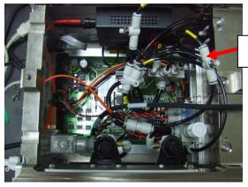
Figure 41: Gradually loosening the knob of the inline flow controller A
