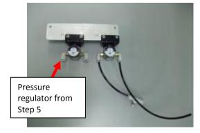
Figure 12: Installing the Pressure Regulator sub-assembly which has been removed in Step 5
