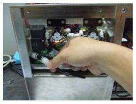
Figure 19: Plugging the M8 tubing end from Step 16
