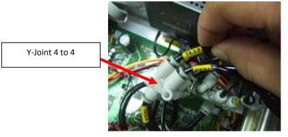
Figure 25: Identifying the tubing with label Y4.3.B
