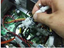
Figure 26: Plugging in the inline flow controller B sub-assembly from the permanent fix kit
