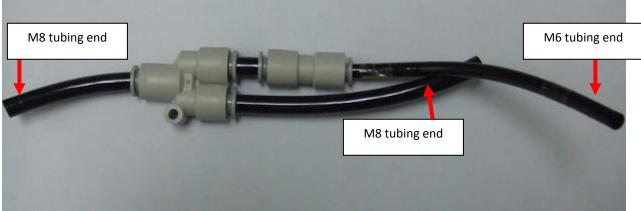
Figure 9: the removal of the existing tubing and fitting assembly
