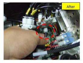
Figure 16: Plugging the M6 tubing end from Y-joint 6 to 6 into the elbow fitting
