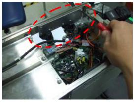
Figure 15: Installing the Pressure regulator mounting sub-assembly from Step 12 onto top extrusion plate
