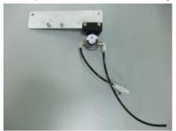
Figure 11: Pressure Regulator Mounting retrieved from the permanent fix kit
