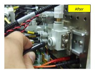
Figure 8 Disconnecting M8 tubing end from the Incoming Port
