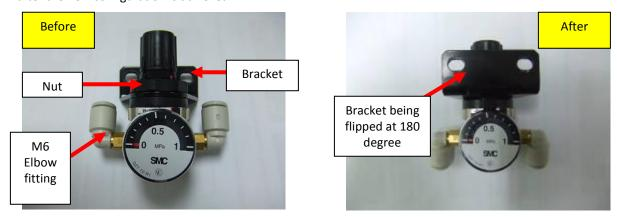
Figure 10: Flipping the pressure regulator to new configuration
