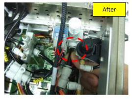
Figure 17: Plugging the M8 tubing end from the straight reducer 8 to 6 into the incoming port
