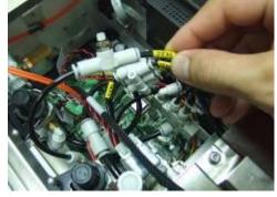
Figure 22: Identifying the inline flow controller A
