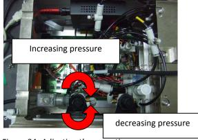
Figure 34: Adjusting the operating pressure
